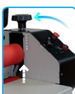
A single elevation control elevates the upper roller, with an indication of the opening on the side. Maximum opening is 5cm. The alignment of the rollers is adjusted during production and guarantees perfect lamination results at all times.
