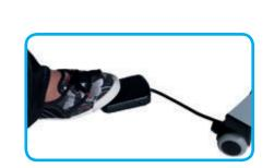
The operator safely drives the machine with a foot pedal.
